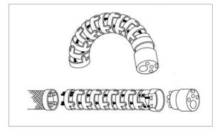
pipes. The wire is threaded through and eye loop on each vertebra down to the distal tip where it is attached. This tension reduces the air space causing the distal tip to bend in that direction. By turning another knob, a wire bends the tips in another direction. A combination of up/down and left/right allows the tip to bend in any direction. By pushing the insertion tube a little, you can steer and advance through most intricate lumens of the body as far as the instrument's length will allow.
