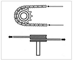
The current Olympus models have replaced the cable and pulley with a chain and sprocket system similar to that of a bicycle. The chain wraps around the sprocket and moves in the direction it is turning. The chain and the angulation wire inside the insertion tube are attached together.
